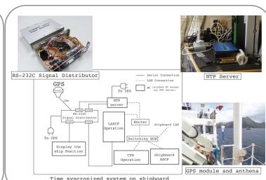
Time synchronized server (NTP server) system. For the time synchronization of analysis equipments such as CTD, LADCP, ship board ADCP, and so on, we developed a low-cost NTP server using GPS with GPS signal distributor. This system achieved a long-time cruise without big trouble.
