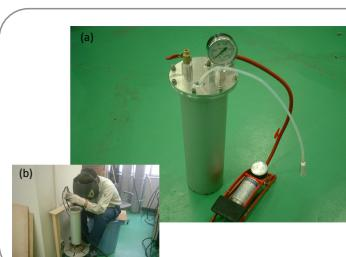
This is an instrument to trap microorganisms in water (requested by Microbial Ecology Group: 400mm in length). This instrument is made in aluminum which is light and easy to carry out for field observations. It compresses a bag of water samples by pumps, and traps the samples in filters through small pipes (a). The aluminum weld was found out the best way for non-leakage of the air (b) by leaking checks.
