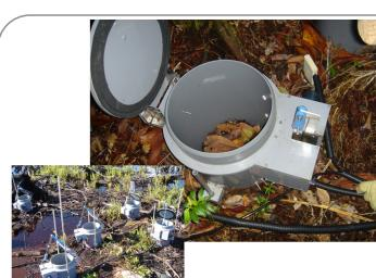
This apparatus is to observe CO<sub>2</sub> efflux from soil or snowpack etc. by measuring the change rate of CO<sub>2</sub> concentration inside the chamber. Technical division have been manufactured nearly 300 chambers with different sizes.
