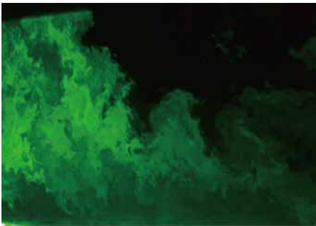
接地境界層における乱流の可視化計測 Image velocimetry of turbulent flow in the atmospheric surface boundary layer
