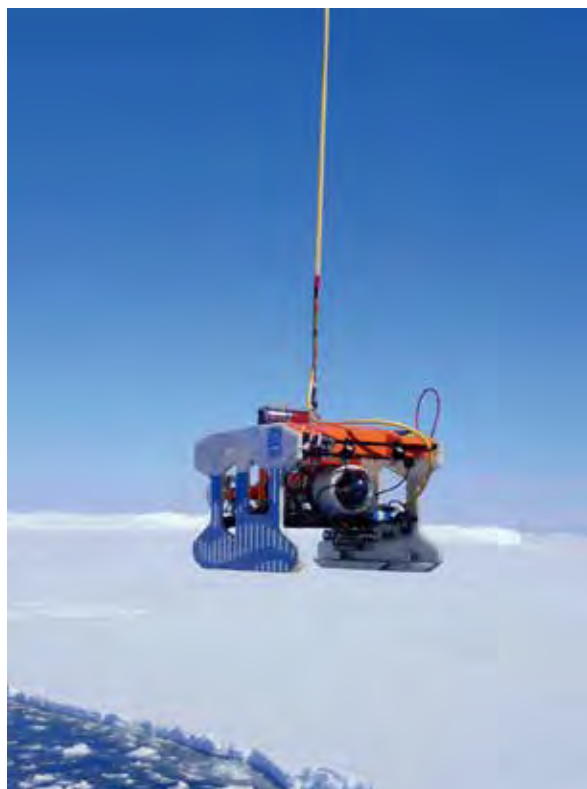
水中無人探査ロボットを用いた南極海海氷下の観測 Observation under Antarctic sea ice by a Remotely Operated Vehicle
