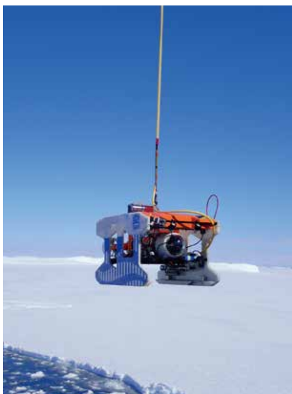
水中無人探査ロボットを用いた南極海海氷下の観測 Under Antarctic sea-ice observation by the Remotely-Operated Vehicle
