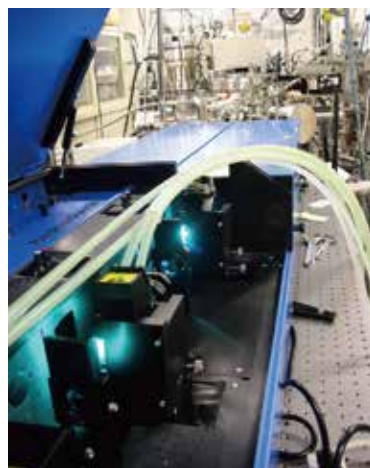
固体表面の原子や分子を調べるための波長可変型色素レーザー A wavelength-tunable dye laser system for the analysis of atoms and molecules adsorbed on the surfaces of solids.
