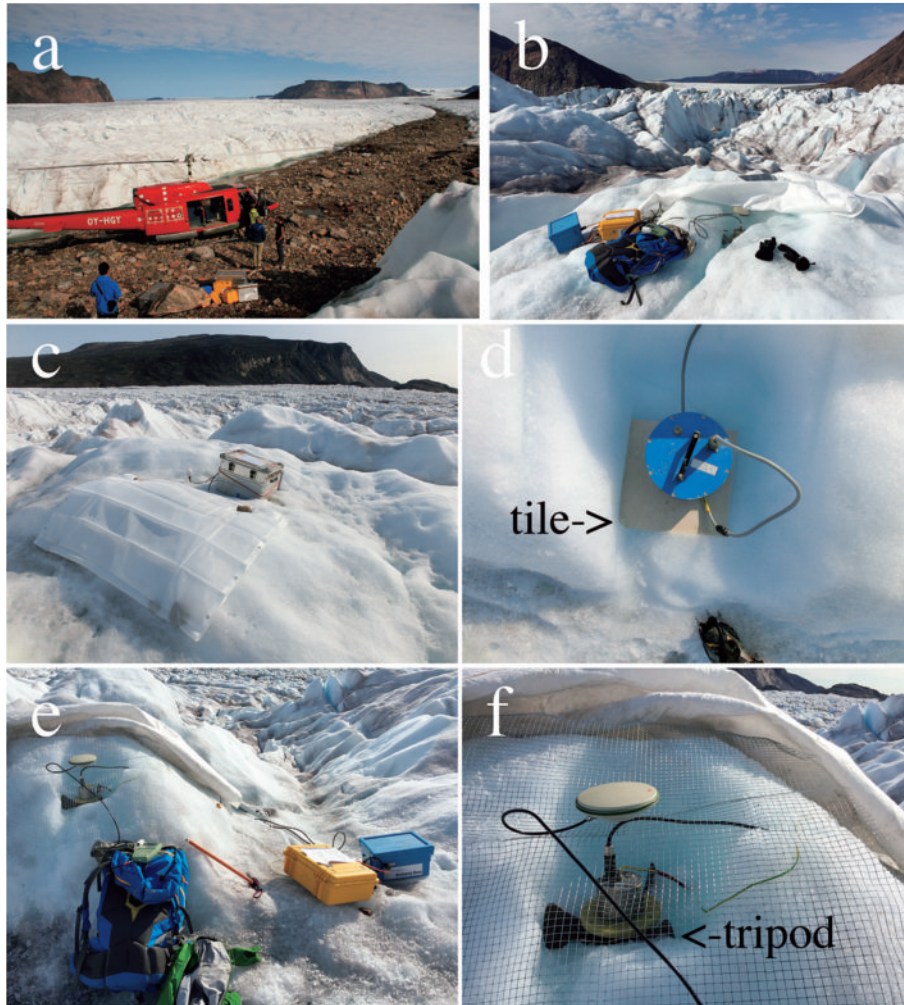
Figure 2 : (a) Staging area for seismic equipment on the central moraine, unloaded from the helicopter. (b) Seismic station IC1. An SP seismometer was screwed to a disk and placed on a metal tripod. Note the drainage channel for removing meltwater from the ice pit. The yellow watertight box contains the Taurus recorder, GPS antenna, and solar panel regulator. This box is connected to one external battery (Cyclon; 12V, 46 Ah) and a solar panel. (c) Seismic station ICC. An LP seismometer was placed in an ice pit and covered with a mesh and protective blanket. The aluminum Zarges box contains the Guralp recorder, battery (Fiamm, 12V, 42 Ah), and solar panel regulator. The solar panel and GPS antenna are located at the sides of the box. (d) LP seismometer at station ICC deployed on a ceramic tile. (e) Seismic station IC2; setup is as for station IC1 — see (b) above. (f) SP seismometer at station IC2, deployed on a metal tripod. Note that the Leica Geosystems dual-frequency GPS antenna is placed into an intentionally formed depression in the mesh so that a consistent measurement position can be obtained. This strategy was also employed at station IC1. Efforts were always made to ensure that other parts of the mesh were kept away from direct contact with the cable.
