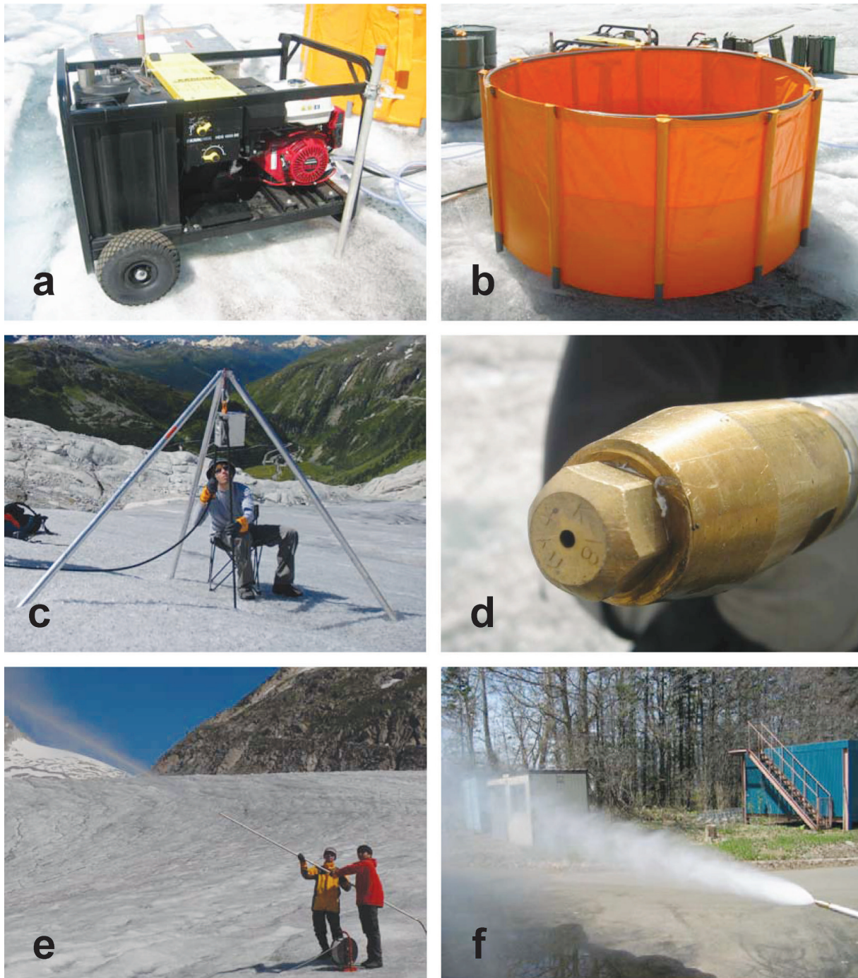
Fig. 3. (a) The high-pressure hot water machine (Kärcher HDS1000BE), (b) the 3000 l water basin, (c) the tripod with its pulley, (d) a jet nozzle mounted at the tip of the drilling stem, (e) a water jet from a 3 m long drilling stem with a straight nozzle, and (f) a water jet from the conic spray nozzle.
