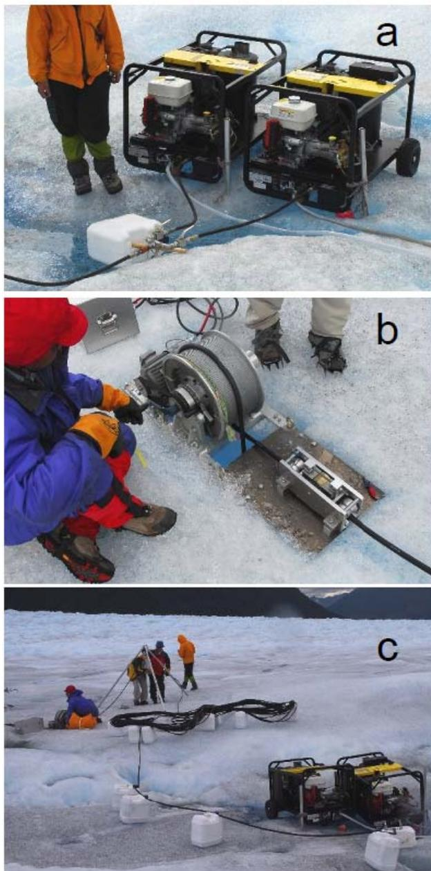
Figure 2. (a) High pressure hot water machines. Hot water discharges through the black pipes, which are combined into one hose with the piping. (b) Winch system with a brake in the lower right. (c) Hot water drilling system set up on Glaciar Perito Moreno. The borehole is at the middle left.
