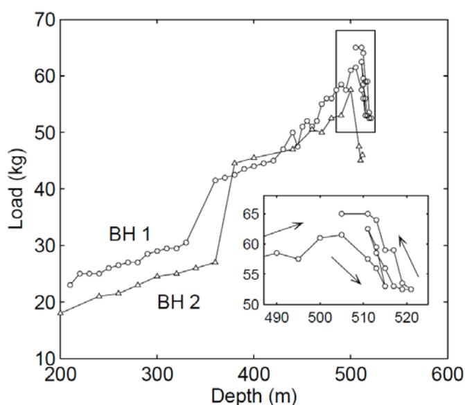
Figure 4. Weight of the drilling hose measured during the drilling of BH1 (○) and BH2 (△). The inset shows details near the bed in BH1.
