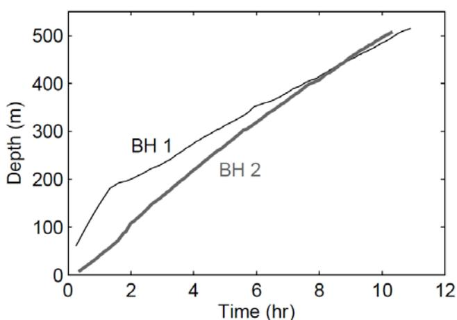
Figure 3. Depth of the boreholes v.s. drilling duration for the drilling of BH1 (black) and BH2 (bold gray).
