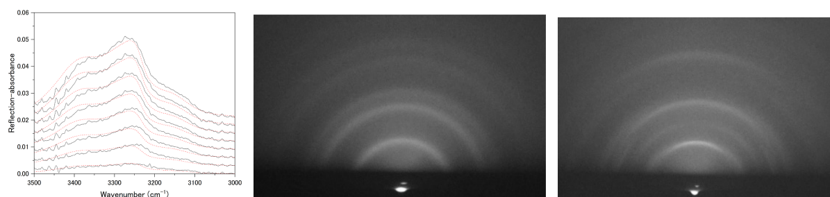
Figure 1: (Left) IRRAS spectra showing OH stretching vibration region for vapor-deposited ice growing at the temperature of 130 K and the water vapor pressure of 2 \times 10^{-6} Pa, recorded between 30 and 240 minutes. The black solid and red dashed lines represent experimental and fitted spectra, respectively. (Center and Right) RHEED patterns of the ice grown for 60 min (6.2 nm) and 420 min (42 nm). Debye-Scherrer rings indicate that the crystal structure of the ice is polycrystalline Ic (Center) and Ih (Right), respectively.
