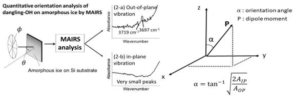
**Figure:** (left) Schematic illustration of IR-MAIRS. IR–MAIRS: Typical single-beam spectra measured at an angle of incidence of 45° at various polarization angles from 0° to 90° in 15° steps, and then extracting the IP and OP spectra by multivariate analysis.
