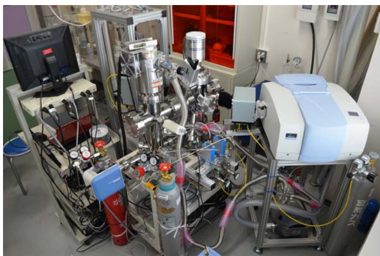
Figure 1: Photo of the newly developed system for catalytic reaction experiment. This system has differential pumping system, a temperature-controlled substrate (26-800 K), FT-IR, two Q-MSs and gas flow controller.
