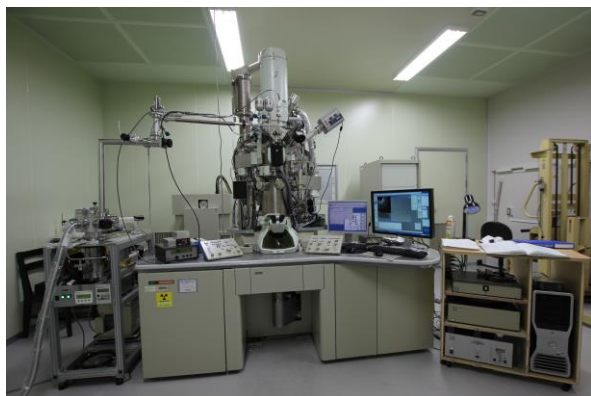
Figure 1: UHV-TEM (left) and UHV-AFM (right).
