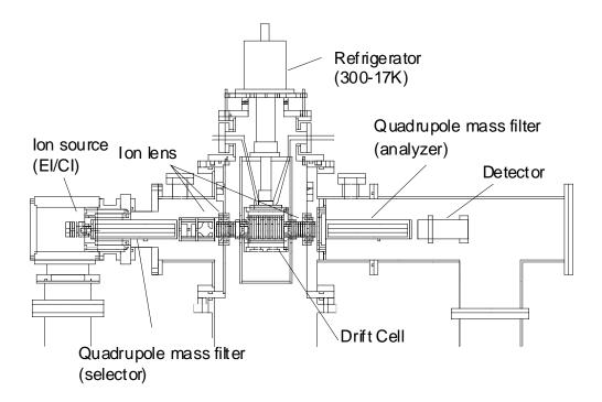
Figure 1: Schematic diagram of the low temperature ion drift tube mass spectrometer.
